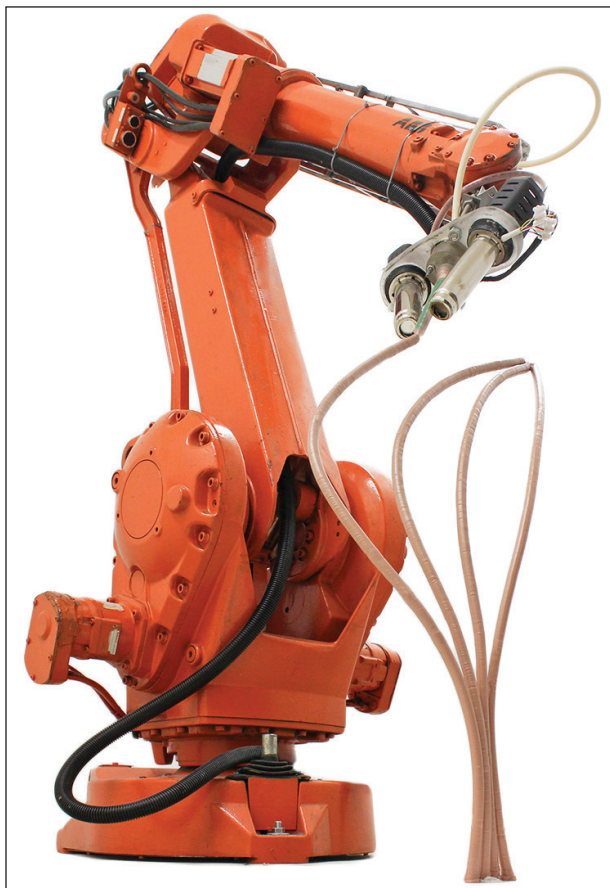
Figure 1.3 Mataerial multi-axis 3-D printer (source: Mataerial home page, accessed April 25, 2017, www.mataerial.com ).
