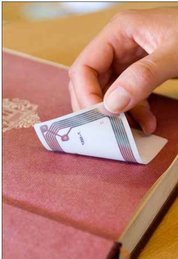
Figure 1.1 48 mm x 80 mm TAGSYS Folio 370-F3 tag. Photo provided courtesy of TAGSYS. See "Folio HF RFID Tags," datasheet, TAGSYS RFID website, 2012, http://tagsysrfid.com/content/download/463/3044/version/3/file/T-M-FolioTags-Datasheet-6Mar2012.pdf .
