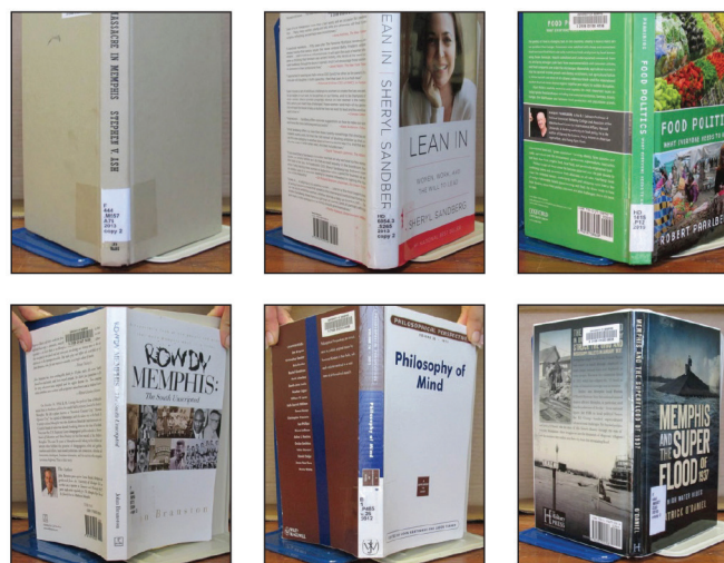
Figure 1. First row, left to right: Plain cloth cover; dust jacket; paper-over-boards (the material covering the boards wraps around the edges and is glued under endpapers). Second row, left to right: paperbacks with publisher-supplied information; paperback with plain cover; Vinabind (the material covering the boards is applied only to the outer surface of the boards; the white edges show the boards underneath the cover).
